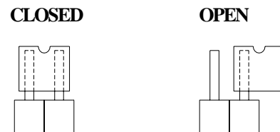
2-pin Jumper (JP1...JP4): graphic example of various setting possibilities
